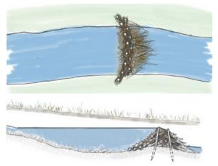
Channel spanning structures create ponding and catch sediment on their upstream side. These ponds provide important habitat during the summer when flow is at its lowest and serve as speed bumps during high flow events, slowing the water and giving the sediment a chance to settle and collect. Ideally structures can raise the water level enough to reconnect to the floodplain allowing floods to dissipate over their floodplain and providing nutrient rich soil to the area.
