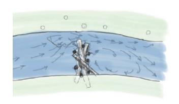
Bank-attached structures are ideal for incised. high flow areas. They don't try to hold back water. Instead, their goal is to redirect water around the structure, encouraging sinuosity and sediment redistribution from the high bank opposite the structure and deposition both in front of the structure and in the eddy behind it. They are crucial for directing sediment back into the channel where it can accrue behind the channel-spanning structures downstream for floodplain connectivity.
